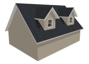
8. Notice there are small gaps in the dormer side walls. This gap is caused by the difference between the position of the knee walls and the point at which the ceiling intersects the roof plane. This location is marked by the black dotted line in floor plan view.
