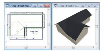
Notice the step in the ridge line. This can be corrected by resizing the lower gable wall. Select the vertical wall to the right of the bottom gable wall and move it to the left 2 feet, reducing the length of the gable wall from 20 to 18 feet. When you are finished, rebuild the roof.
