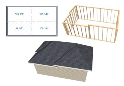
If you generate a roof and it seems to be more complicated and has more roof planes than it should, take a look at the ceiling heights of the rooms in the plan. Often, the correct way to create a lowered ceiling condition will be to set the ceiling at the default height create a lowered Ceiling Finish. See "Lowered Ceilings" on page 128 of the Reference Manual.
