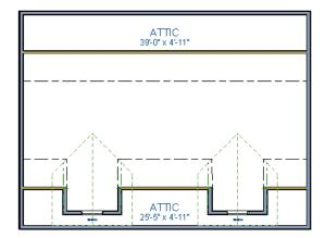
9. Select each of the knee walls and move them back so that they are in alignment with the ceiling plane. The walls will snap into position when they are close to the ceiling lines.
