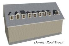
• Specify the **Pitch** of the dormer roof planes. Initially, the default dormer pitch matches the roof pitch for all dormer roof types except Shed, which has a default 3 in 12 pitch. For Gambrel and Mansard types, this applies to the lowest, or eave, roof planes.
