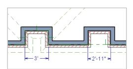
The Roof Overhang is measured horizontally from the exterior surface of the wall's framing layer to the end of the top of the rafter. It does not include gutters, sheathing or siding.
