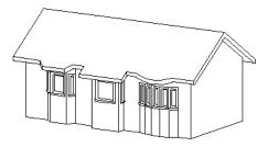
For this roof style, the ceiling heights of the window unit and the adjacent room must be the same. If you lower the ceiling of the window unit and then build the roof, a lower hip roof over the window is created. See "Floors and Ceilings" on page 173.
