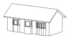
With this option the bay, box, or bow windows is tucked under the roof eave. You may find it helpful to increase the width of the eaves. See "Roof Tab" on page 206.
