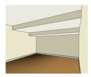
In a situation like this, a Lowered Ceiling can be used to cover "steps" made by different floor heights on the floor above. See "General Tab" on page 143. To ensure that steps in floor and ceiling platforms have solid sides, define their room areas using Invisible Railings.
