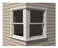
To create a corner window, first create the desired window on each side of the corner. The header height and the sill height of both windows must be the same. To move a window all the way into a corner, check Ignore Casing for Opening Resize in the Plan Defaults dialog. See "General Plan Defaults Dialog" on page 51.
